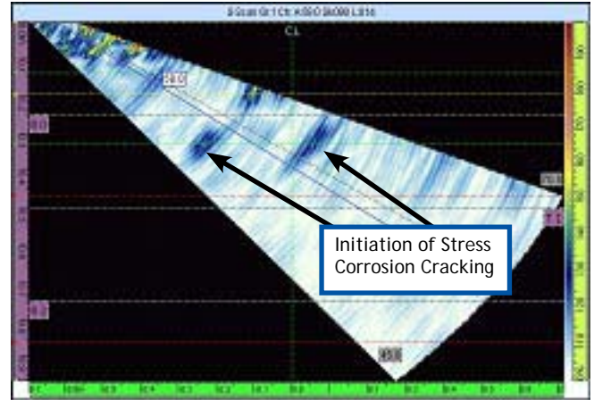
Typical responses from a cracked specimen are shown. The figure above shows the initiation of stress corrosion cracking on the ID of the piping.
