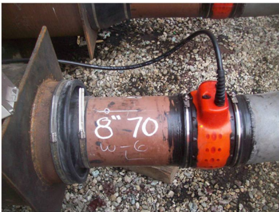
Permanently installed GUL monitor eliminates future digs and provides accurate information regarding Asset Integrity.
