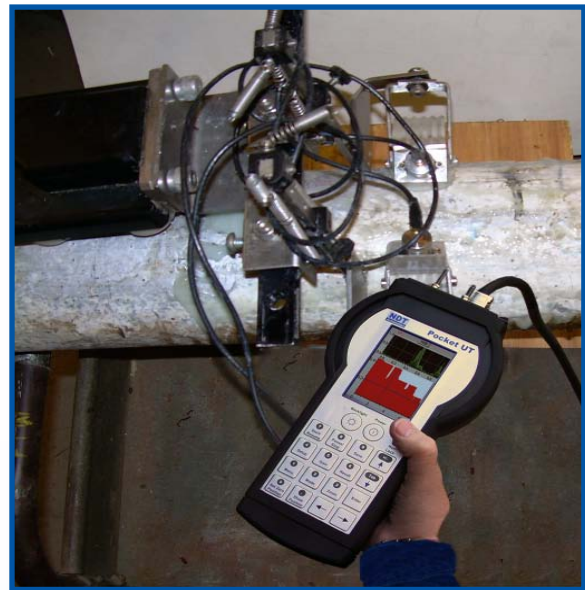
Figure 1. MISTRAS designed and manufactured Pocket UT System with portable flexible Bridge Assembly to fit many pipe sizes used for Touch Point Corrosion™ Inspection
