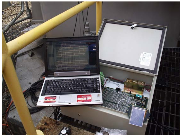
Figure 4. Configuration of the Sensor Highway II™ System via a Laptop
