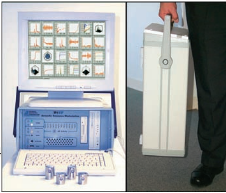
Figure 5: Compact, portable, 24-channel DiSP-24 AE Workstation.
