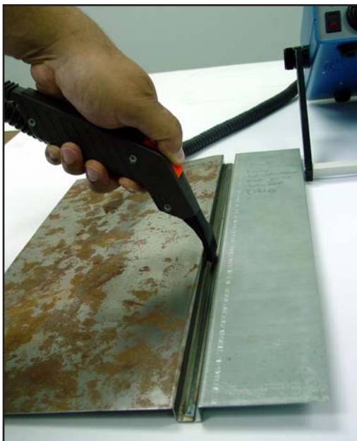
Figure 1. M100A shown measuring the quality of a laser seam weld.
