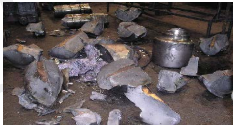
Catastrophic Roll Failure
