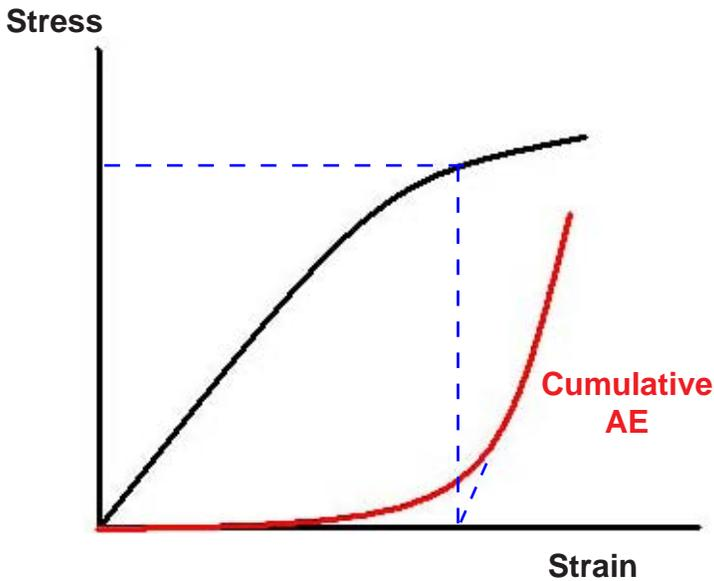
Figure 3. Stress-Strain (Black) Response of Composites Compared to Cumulative AE (Red)
