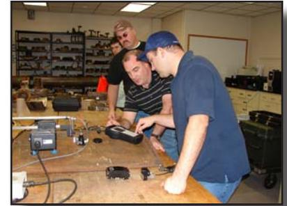
The input of customers, like Nyholt, has allowed the Pocket UT to evolve into a system that is necessary in the location and documentation of corrosion in piping systems and vessels. With the multiple scanners available from MISTRAS and other manufacturers around the country, BP has found a versatile system for many applications.
