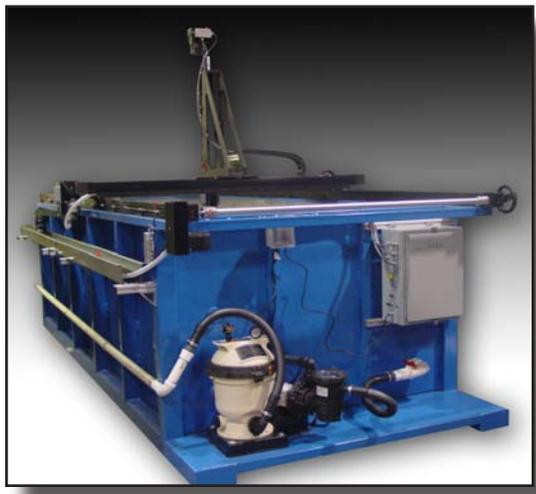
At the left we have a 16' long, 3 axis industrial scanner which was delivered to a major NDT aerospace composites inspection company. The customer needed a precise yet high speed inspection with little user intervention. The system is fully stainless for all surfaces in contact with water and includes a through transmission squirter adapter for honeycomb laminates.
