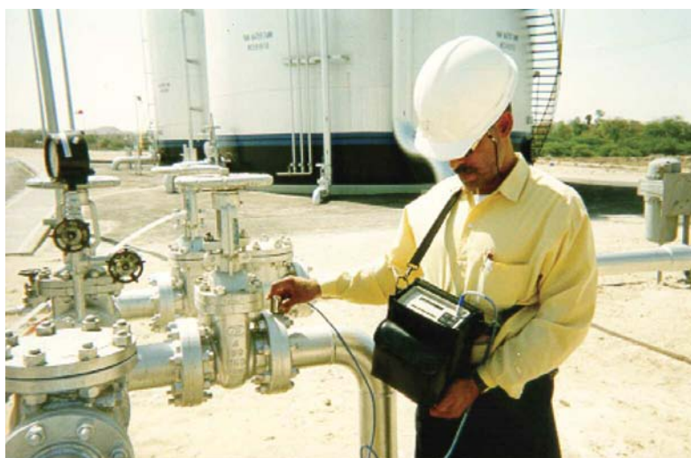
Figure 5. Piezoelectric elements used in many AE instruments are capable of generating large voltage spikes. AE instruments should be verified intrinsically safe before use in a plant or hazardous area.
