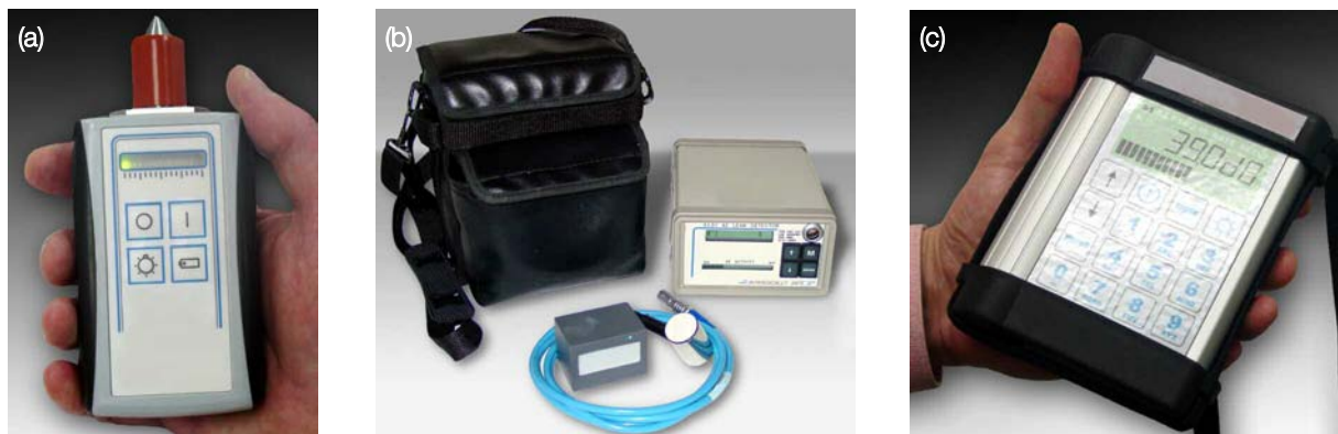
Figure 4. Leak detection systems: (a) handheld, high frequency, nonquantification system for spotting leaks, (b) system with quantification capabilities and (c) handheld system with quantification capabilities.
