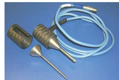
Figure 7. Acoustic emission sensor and waveguide for high temperature valves.
