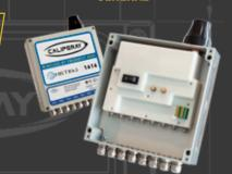
Receiver: 20-70dB Gain Bandwidth: 1MHz to 9MHz
