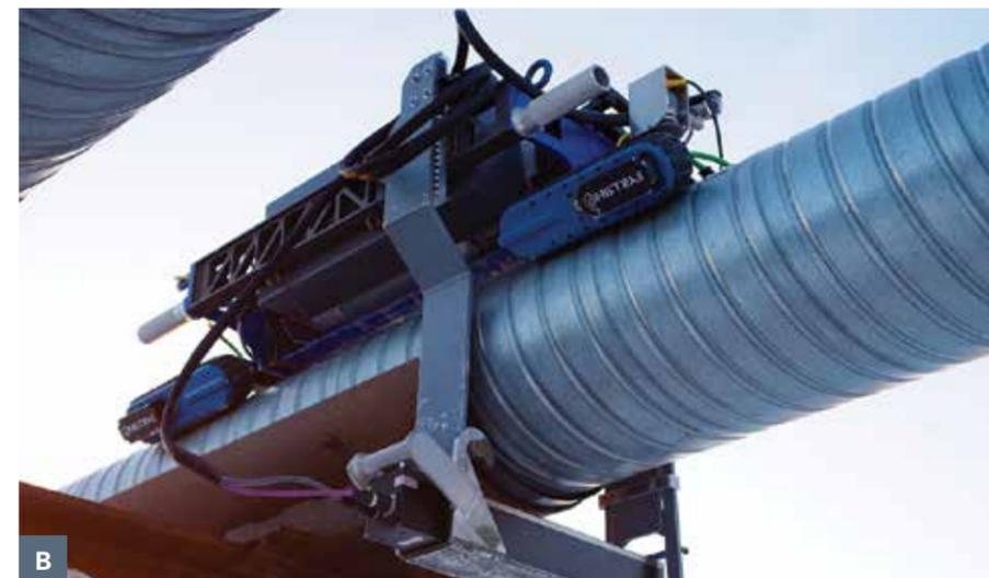
**A:** The PIMS remotely informs pipeline operators of asset conditions from difficult-to-access or hazardous locations. Mistras' **B:** ART Crawler can be used to detect corrosion under insulation.
