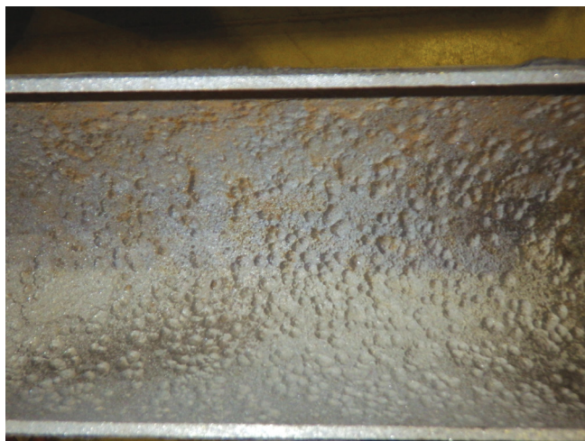
Figure 3. Neural networks can be trained to recognise and size thousands of real-life anomaly types, including pitting and corrosion.
