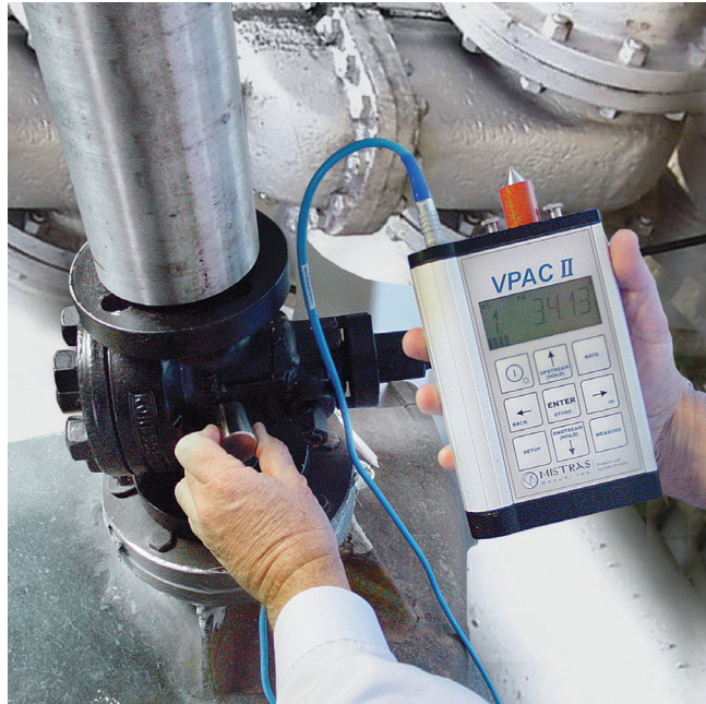
Figure 1. A technician performs a valve test using the handheld MISTRAS VPAC™II. With preloaded valve routes and properties, the leak detection system is able to provide on-board leak rate estimates during a test.
