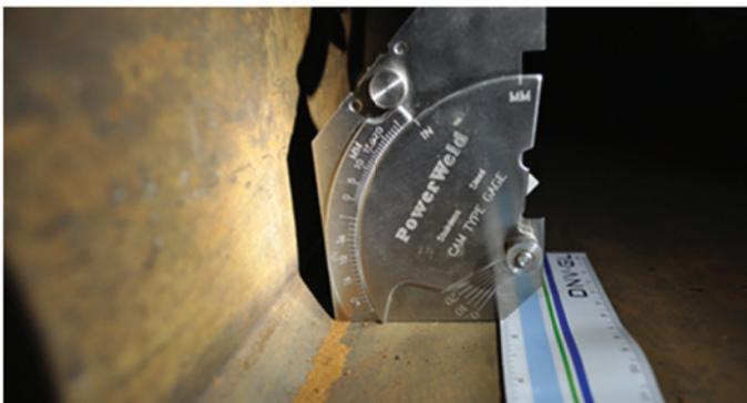
**Figure 3.** Corner-weld as-built view [4].
