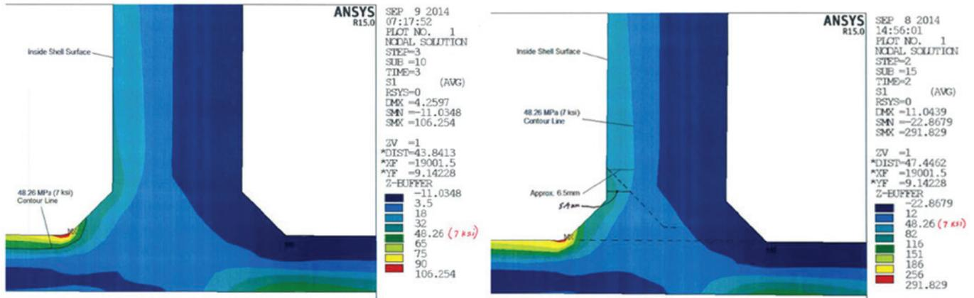
**Figure 7.** Stress States at Corner-weld. Values reported in MPa. Left: Normal Operating Liquid Level. Right: Design Liquid Level [6].
