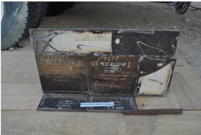
Figure 5. As-built mock-up for PAUT scan plan and calibration [4].
