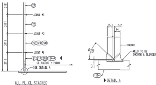
**Figure 2.** Corner-weld Conceptual Design [3].
