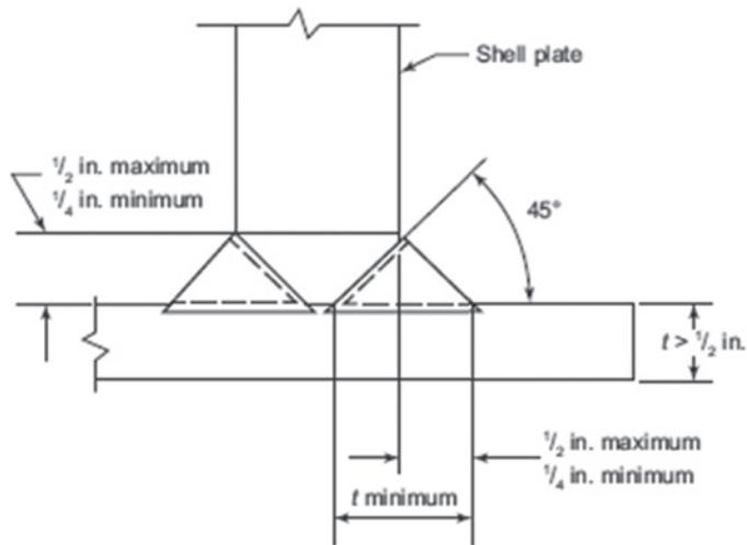
**Figure 1.** Double Fillet-groove Weld for Bottoms Greater than Half-inch (Source: API Standard 620, Figure 5-3) [1].
