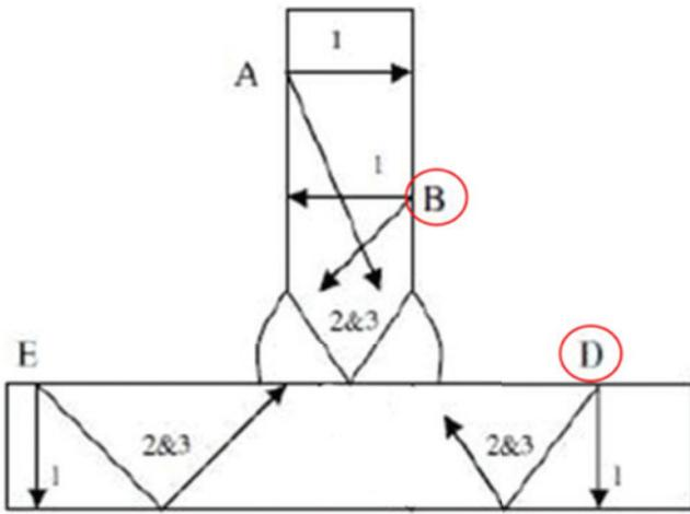
Figure 4. Transducer Position for PAUT Scan Plan [4].
