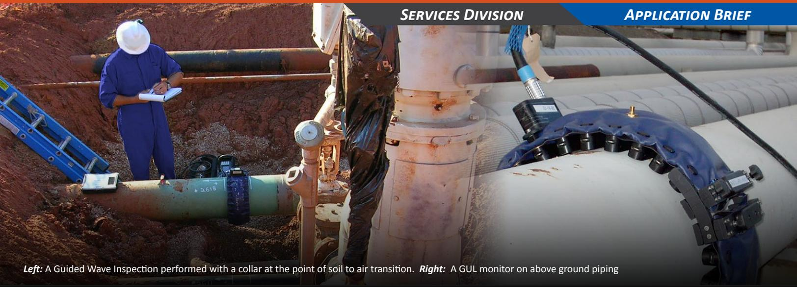
**Left:** A Guided Wave Inspection performed with a collar at the point of soil to air transition. **Right:** A GUL monitor on above ground piping
