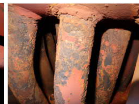
4. Erosion & Corrosion Damage on VIP2 Tubes (Blue) Due to HP2-1 Tube Water Jet Leak
