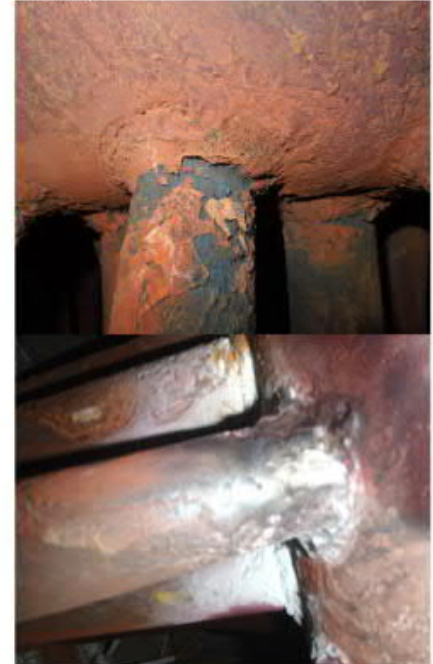
Erosion & Corrosion Damage (Blue) on Header 27 Due to HP2-1 Tube No: 5 Water Jet Leak
