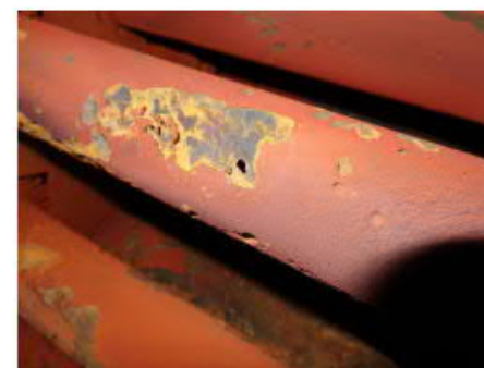
3. Hole on VIP2 tube (Red) Due to HP2-1 Tube Leak Water Jet Erosion
