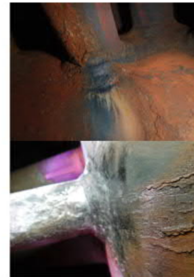
Primary Leak Source - Crack Facing Header 27 at Front Row Tube No. 5 Joint of Header 29 – See Water Jet Leak Area Marks
