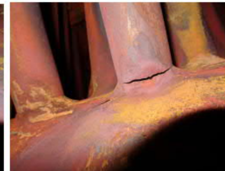
1. Full Circumference Cracked Tube No. 3 (Red) & 2. Partially Cracked Tube No.5 (Red) at Tube Joint on Header 29 as Primary Source of Water Jet Leak
