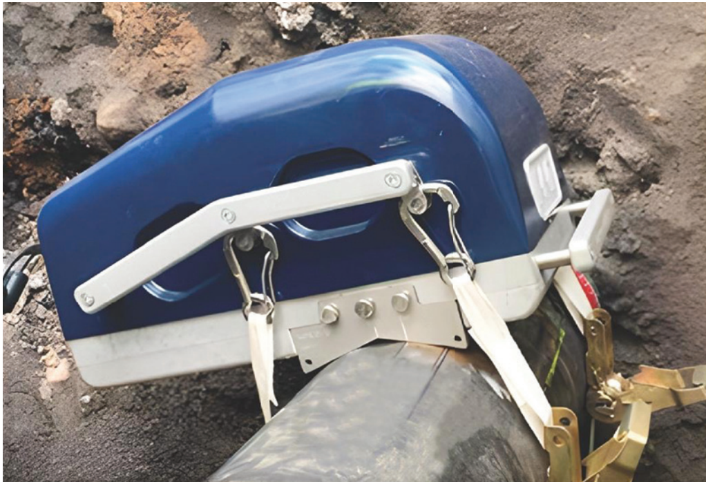
Figure 2. Advanced hardness, strength, and ductility (HSD) services can provide TVC records for missing integrity data to allow full utilization of the maximum allowable operating pressure (MAOP).
