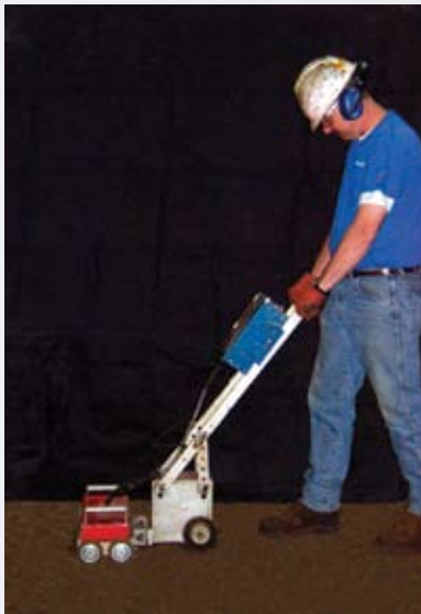
Magnetic Flux Exclusion inspection being performed during an Out-of-Service inspection to determine potential loss of material on the tank floor.
