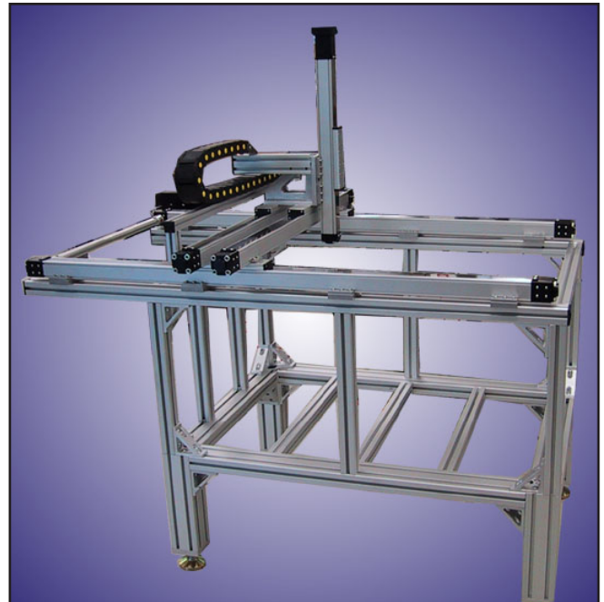
Figure 2: Overall view of frame assembly
