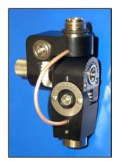
The positioning of the ultrasonic transducer is smooth and responsive, which is accomplished with precision worm gears through manual knobs that allow angular motion of > +/- 93° (gimbal axis, front to back) and +/-49° (swivel axis, right to left). By tuning the position of the transducer, you gain
