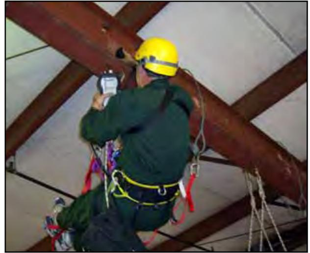
*An area of interest was confirmed to be badly corroded after being scanned with the Pocket UT and Z-Scan.*
