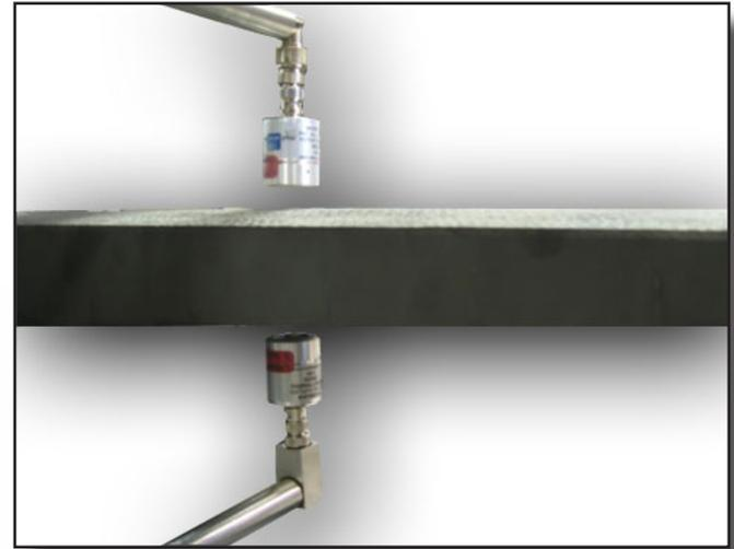
*Composite Sample with Non-Contact, Through-Transmission Ultrasonic Testing*
