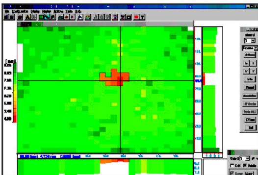
Figure 2: : C-Scan and B-Scans of Elbow showing flat-bottom hole (red).
