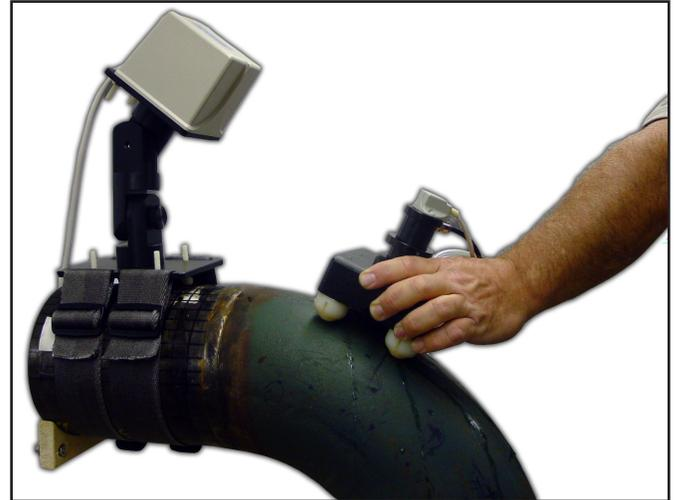
Figure 1: Free Motion Scanner on the curve of an elbow
