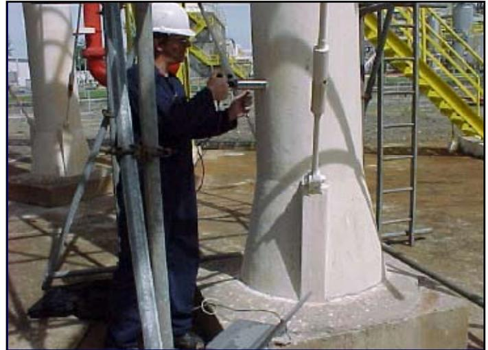
and the leg, which allows water to be present and cause corrosion. The test is usually carried out on a 200mm grid, each point test taking a few seconds. If bonding is good, then corrosion between the leg and protection is not possible. The impact-echo method uses a special transducer that is connected to a signal processor and notebook computer to analyse the acoustic response to mechanical impact of a known controlled duration.
