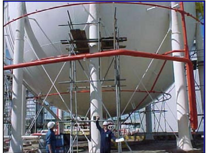
corrosion sensors are mounted near the areas where water ingress is possible. They detect Acoustic Emission coming from active corrosion, a technique used routinely to test process plant and tank floors. Follow-up inspection is required to assess the extent of damage when active corrosion is identified.
