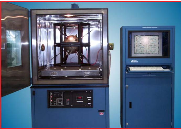
The Halon Bottle Recertification System has a stainless steel, roll out shelf capable of holding Halon bottle and fixture up to 200 lbs.
