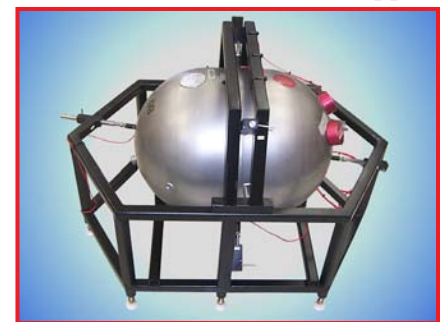
The Halon bottle fixture has a welded steel frame with flip-open top clamshell. 6 spring-loaded sensor rods (12" long) with sensors and coupling pad at end make contact with the Halon bottle when placed in the fixture.
