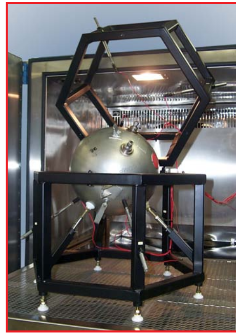
Two fixtures are provided to accommodate to spherical or cylindrical halon bottles.
