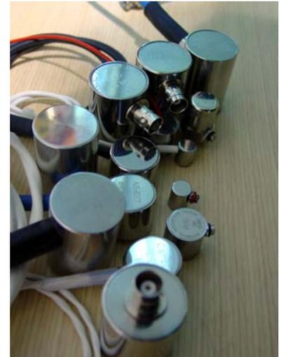
which began in 1968. Our sensors actually “listen” to processes to detect AE activity. In all applications, AE sensors are vital links between the test and the analysis instrumentation. Their performance is critical to the success of every test. They are available in various sizes, shapes, frequency and temperature ranges, and packaging styles to meet the diverse needs of the application and environment.
