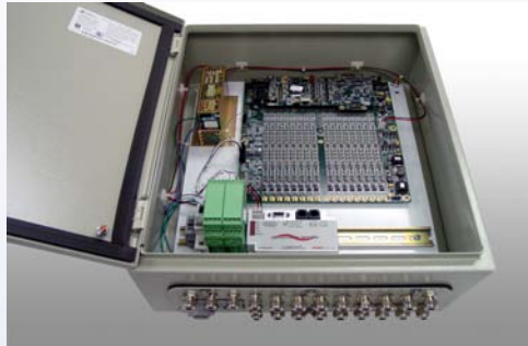
The AE Sensor Highway II monitors the effectiveness of repairs/retrofits
