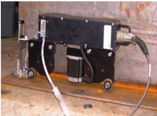
**FIGURE 6B. GUIDED WAVE SCANNING HEAD**
