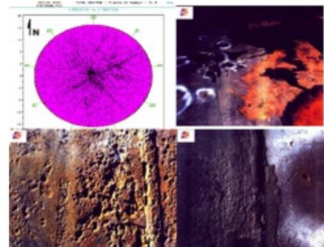
AE testing has proven to be very effective at identifying active corrosion on carbon steel tank floors. Corrosion characteristics are different in other metals such as stainless steel, however. The AE tank floor test is intended to provide a general condition assessment and therefore, it is limited to carbon steel floors. In addition, there are some products, like asphalt, that inhibit the propagation of the signal so they are typically tested under a best effort scenario.
