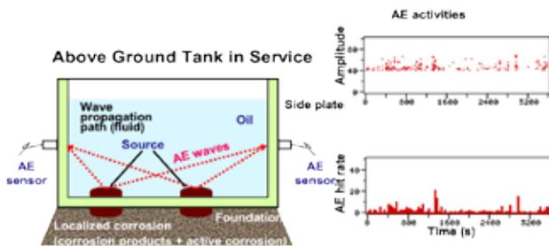
When a tank floor is being tested, the intent is to detect and analyze AE signals from active corrosion. In the field, there are other potential sources of signals that are not related to corrosion. Roof movements, pipe born noise, condensation, particle impact, and valve leakage are some of these. Precautions must be taken so as not to include these noise sources in the final evaluation, otherwise an incorrect determination might be made.
