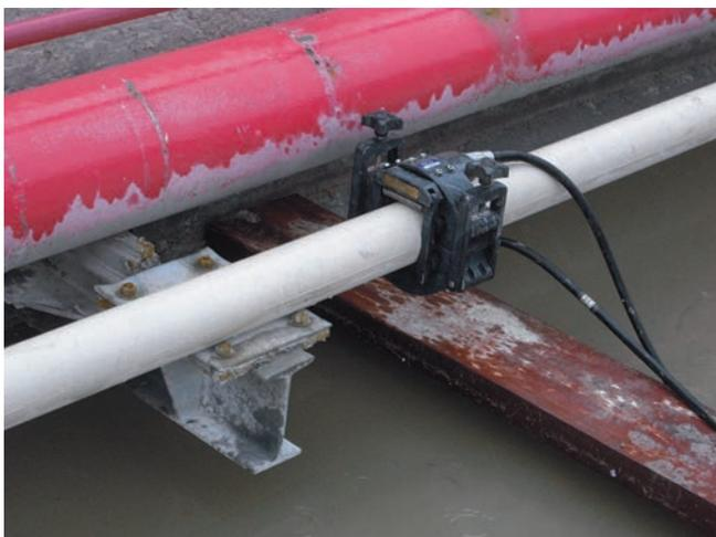
Figure 5. Testing of inaccessible pipes in a river crossing in Rio Grande, Brazil.
