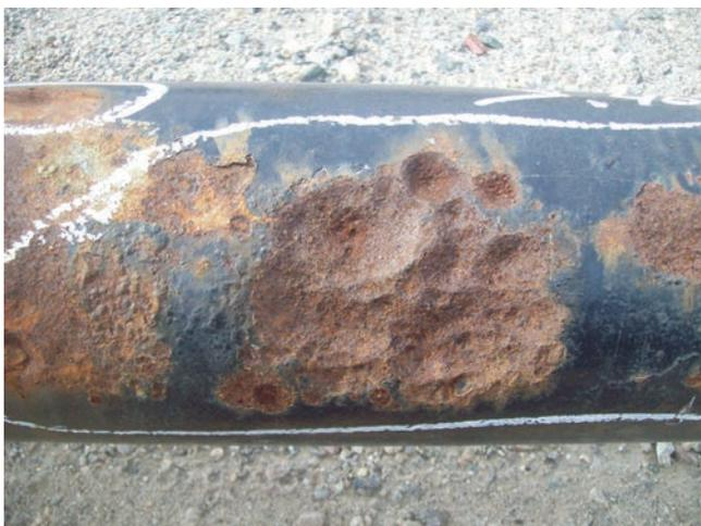
Figure 7b. Discontinuity found with GW in about 8 m of the ring position in a positive direction.
