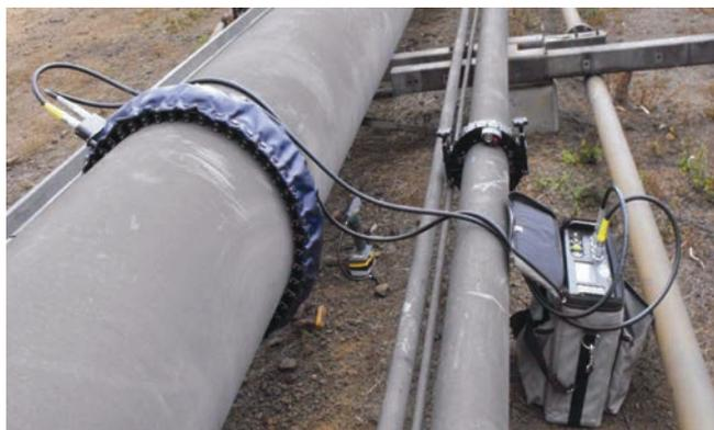
Figure 2. Typical test configuration with test ring and GW equipment from Guided Ultrasonics Ltd. There are several different types and models of test rings, from diameters DN 25 - 1500.
