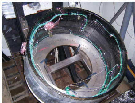
A “softwall” jet engine fan containment case prototype is fully instrumented prior to a blade-out ballistic test. Three types of SHM technologies were employed during the test — including a nanogrid, accelerometers and the intrinsic conductivity of the carbon fiber itself.
