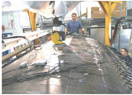
An FAA-sponsored study on curved honeycomb-cored panels showed that acoustic emission (AE) monitoring is a reliable method for locating damage initiation sites and for tracking crack progression.
